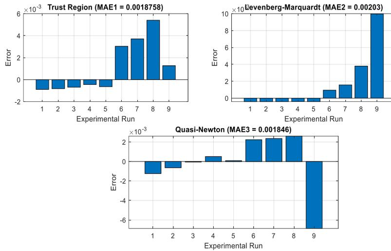
Fig. 8: Residual error spread attained with Quasi-newton in comparison with other techniques during parametric solar cell identification using experimental data 3
