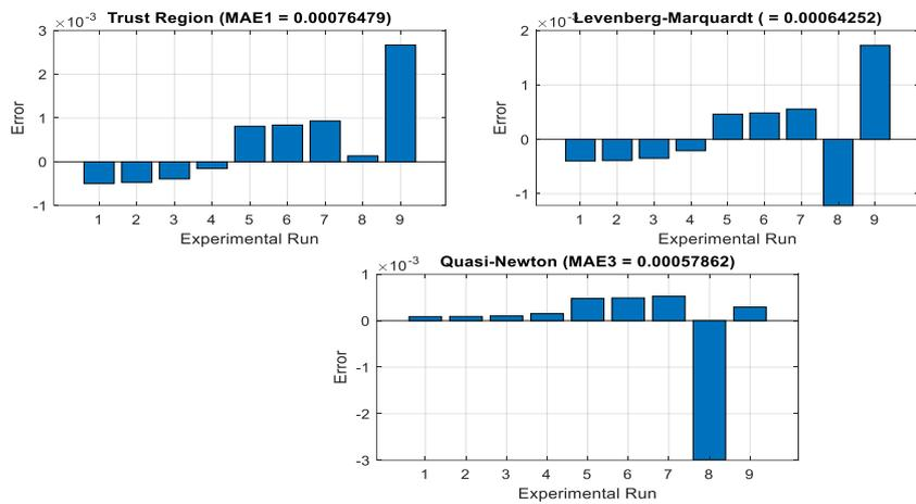
Fig. 6: Residual error spread attained with Quasi-newton in comparison with other techniques during parametric solar cell identification using experimental data 1
