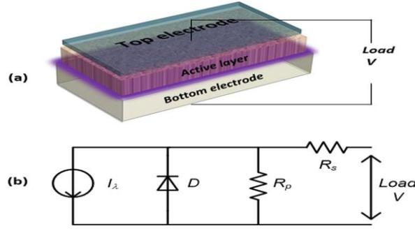
Fig1: depicts the prototype structure of solar cells, with its typical  $I$ - $V$  characteristic curves
