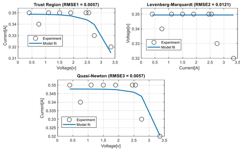
Fig. 5: Fitting accuracy attained with Quasi-newton in comparison with other techniques using Experimental data 1
