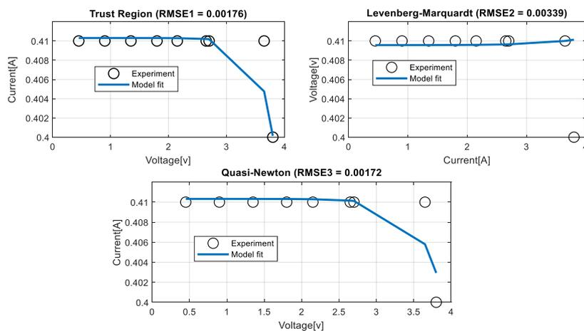
Fig. 4: Fitting accuracy attained with Quasi-newton in comparison with other techniques using Experimental data 2
