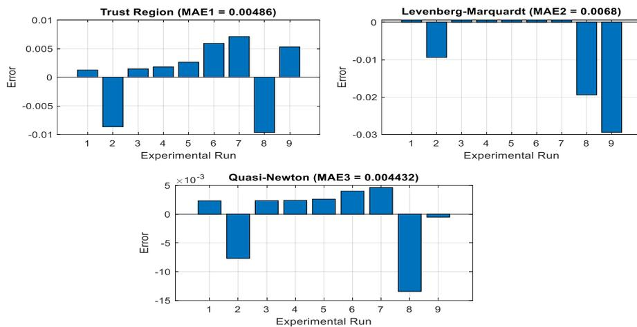
Fig. 8: Residual error spread attained with Quasi-newton in comparison with other techniques during parametric solar cell identification using experimental data 2
